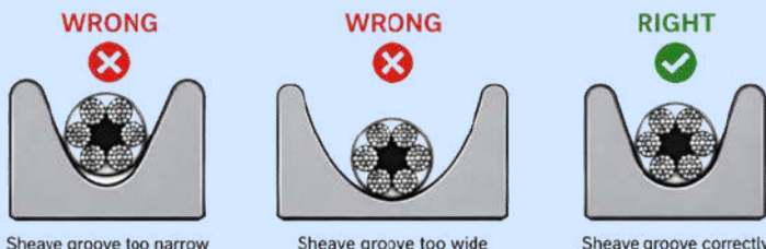
Sheave groove too narrow
